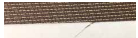
Fiberglass fabric with Fraying
